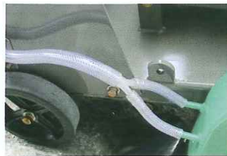
double water pipe for cooling both sides of blade
