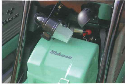
Mikasa cyclone series(MVH-207 ~ 406 with Yanmar diesel engine) Cyclone pre-cleaner increase filterability dramatically! Most suitable for harsh environment
